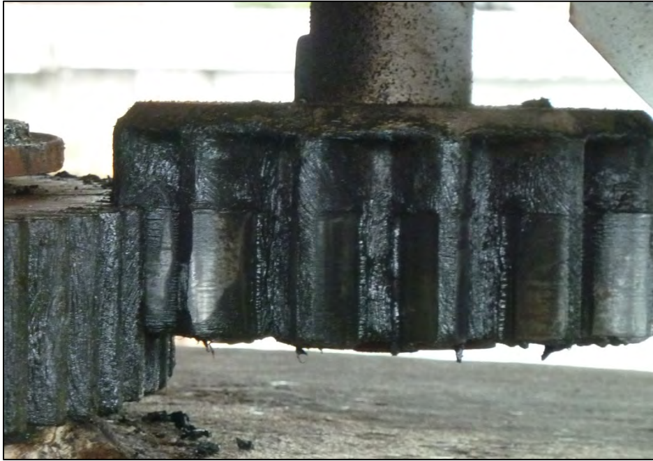
Photo 23 – Emergency Drive Pinion: About 60% engagement with Emergency Drive Rack.
