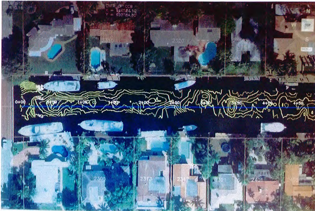
Typical canal bottom survey contour elevations (Picture 13)
